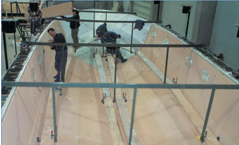
The use of infusion molding for the manufacture of boat hulls, decks and superstructures has grown rapidly in the last few years. Today, a significant number of production boat builders around the world are either using the process or are seriously investigating its value.
