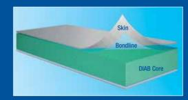
The DIAB sandwich concept increases structural performance while optimizing weight. A sandwich consists of two high strength skins or facings separated by a core material. The skins take up the bending stresses and give the structure a hard wearing surface. The light DIAB core absorbs the shear stresses and distributes them over a larger area.
