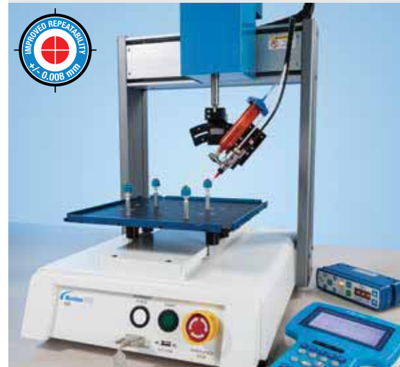
R Series makes 4-axis dispensing automation easy.
