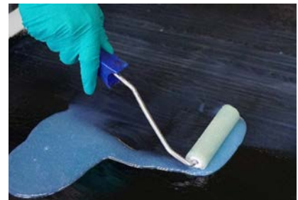
Roller application of SikaBiresin CR169 thix
