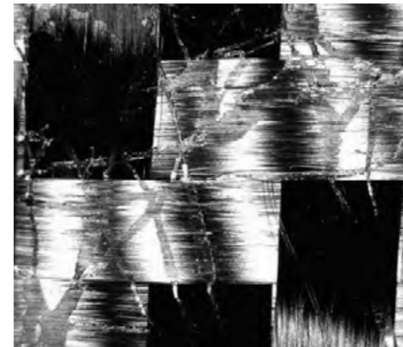
3K Carbon fabric Ref. GG 200 T – 193 g/m 2 | 2x2 Twill weave
