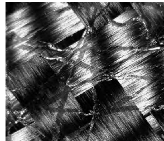
12K Carbon fabric Ref. GG 428 T – 428 g/m 2 | 2x2 Twill weave
